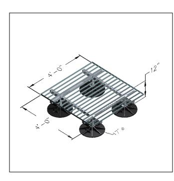
**HV0404L** – **Lightweight Equipment Platform** – Is designed specifically for use on rooftop without adhesive, roof penetrations, flashings or damage to roofing system. Designed to support lightweight HVAC units or transformers. The height of the platform is adjustable to 12" H with adjustable legs. Custom heights are available.
