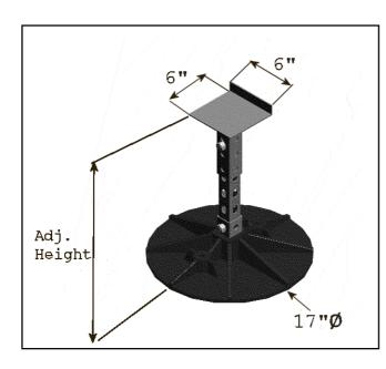
**SS1000E** – **Equipment Support** – Is designed specifically for use on rooftop without adhesive, roof penetrations, flashings or damage to roofing system. Designed to support light-weight HVAC equipment with 6" X 6" galvanized steel support bracket. Height is telescopic to 18". When equipment requires corner supports, use **SS1000EC** as an alternative. Weight disbursed over 227 sq. in. per support.
