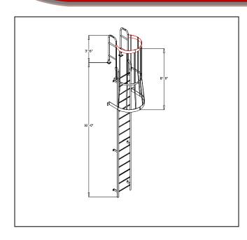
**ASP1602LC** – **Ladder with Safety Cage** – Is designed to be used where a fixed ladder with a walk-thru guardrail is required. Ladder is designed for use where heights require a safety cage for protection. Designed to bolt directly to any ASP Elevated Platform or to structures where fixed ladder is required.
